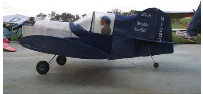
Ken's 1/4 scale model of the Ray Stits "World's Smallest" aeroplane flies quite well on a OS .15. Model needs power on for landing as the glide angle is very steep with the tiny wing.
