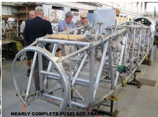
NEARLY COMPLETE FUSELAGE FRAME
